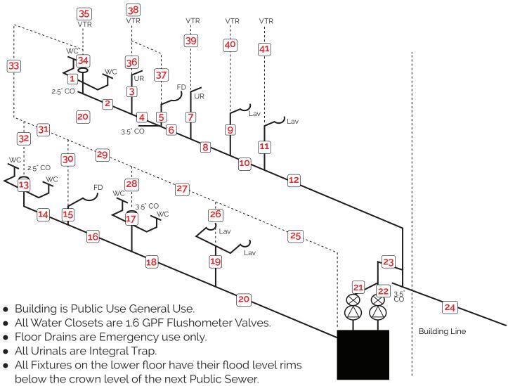
• Sewage Pumps operate alternately and independently but not simultaneously. Each pump discharges 20 GPM.
